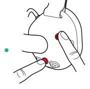
3: The status LED flashes green when connection is successful. If it does not, repeat the pairing process.
